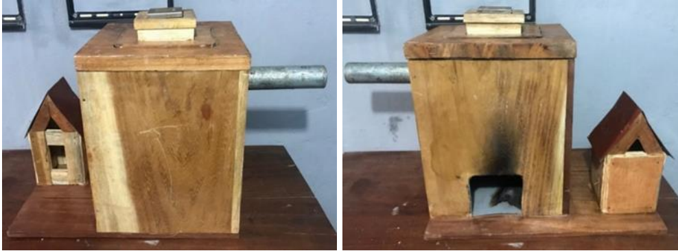
Figure 4. Manufactured thermoelectric system
