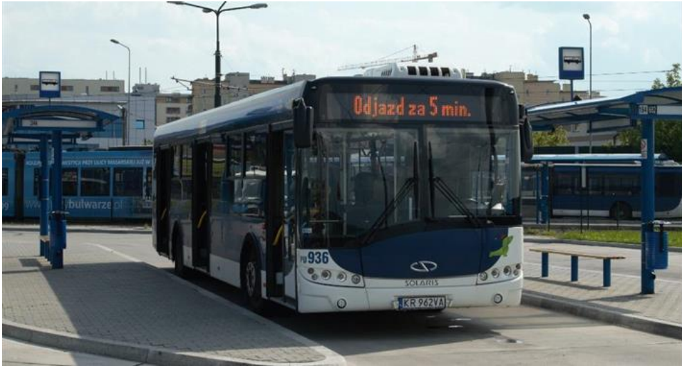
Figure 3: Low-floor Solaris Urbino 12 bus. Buses of this type are now the standard across Europe. ( phot. M.Bis )
