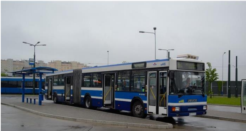
Figure 2: Partially low-floor Jelcz M181MB bus. Buses of this type are being phased out of operation in Poland. ( Phot. M.Bis )
