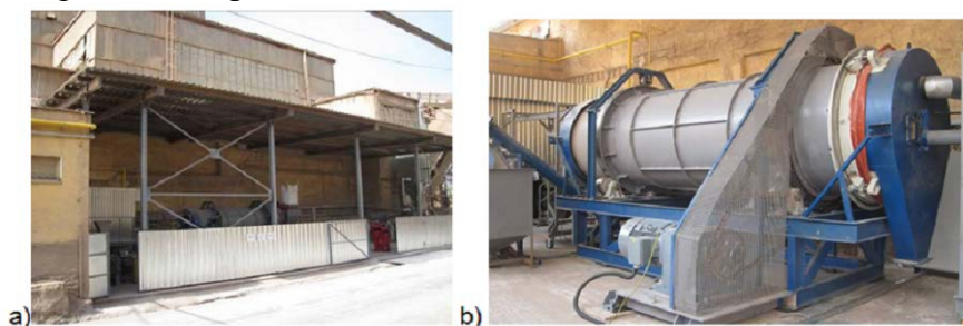
Fig. 7 Pilot high-revolution rotary furnace a) workplace b) furnace 2.1 Experimental verification
