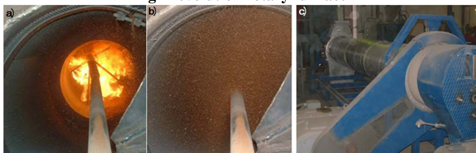
Fig. 6 An inside look into the high-revolution rotary furnace a) low revolutions b) standard operation c) pilot plant equipment
