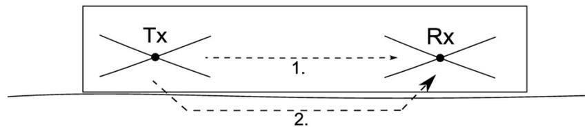
**Figure 1.** Individual components of direct signal. Where Tx is transmitter antenna, Rx is receiver antenna, 1. – signal that travels through air and 2. – signal that travels along ground surface.
