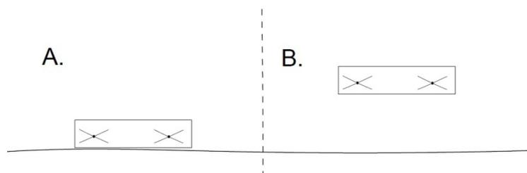
**Figure 2.** *Move out correction* determination experiment. A – initial position of antenna. B – antenna position in the end of experiment.
