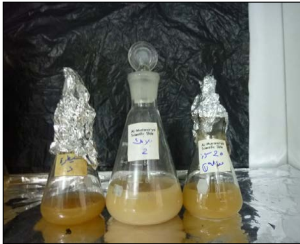
Figure(1): left tube Lactobacillus crispatus in MRS broth without TIO 2 taken as control (B) right tube with bacteria and TIO 2 (0.025 mM) while middle tube is blank TIO 2 and MRS broth only.
