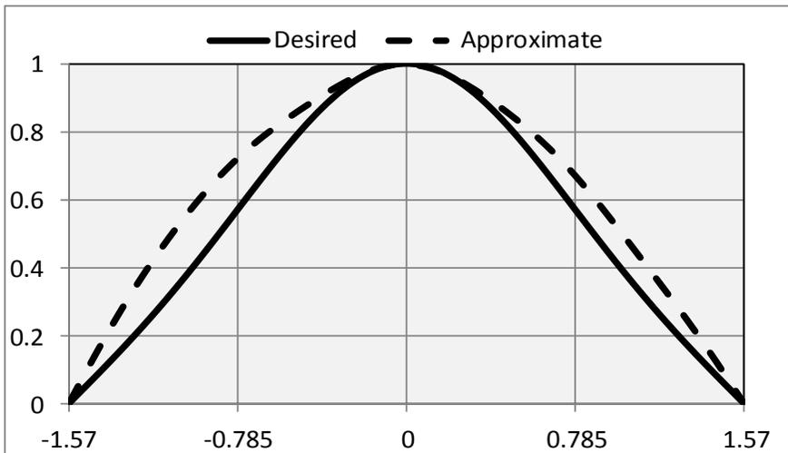
Fig. 2. Amplitude radiation pattern for the undisturbed internal sources  $F_{oi}(\theta, \varphi)$  and the approximate with the auxiliary sources table1.
