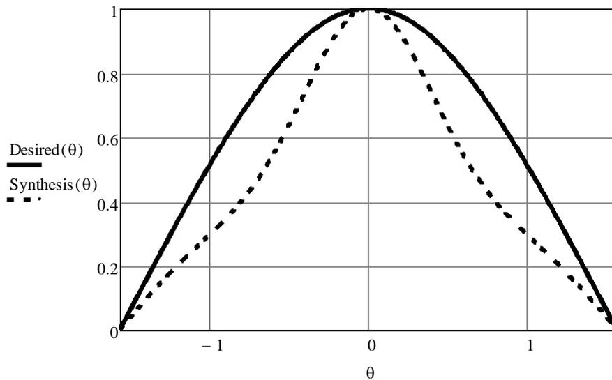
Fig. 6. Normalized radiation pattern desired and synthesis in E-plane
