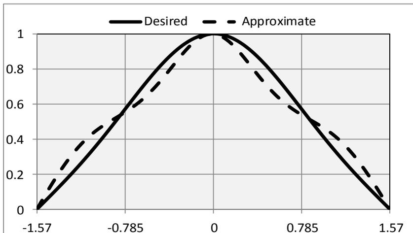
Fig. 3. Amplitude radiation pattern for the undisturbed internal sources  $F_{oi}(\theta, \varphi)$  and the approximate with the auxiliary sources table2.
