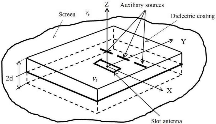
Fig. 1. Slot antenna with a dielectric coating.
