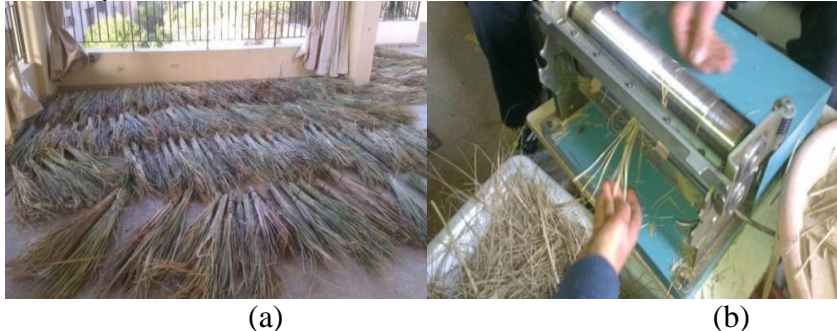
Fig. 2: (a) Dried Fan Palm Leaves, (b) Hand-made Machine for Cutting Fibers
