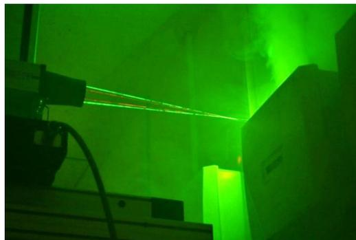
**Fig. 4.** Measuring airflow velocity near an exhaust vent with the two-component LDA system. Vaporized propylene glycol is used for particle seeding.
