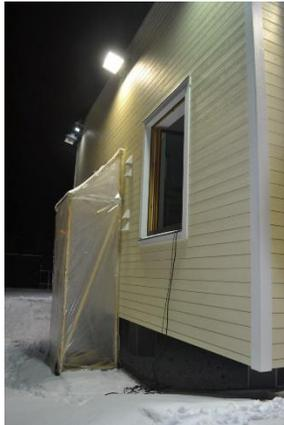
**Fig. 5.** Buffer chamber for a constant supply of seeding particles, connected to the intake of the ventilation unit.
