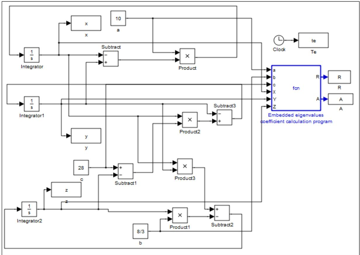
**Figure 1:** Lorenz MATLAB/SIMULINK chaos model
