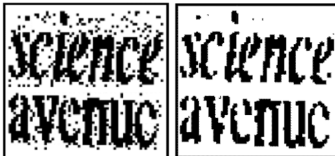
Figure 1. Left: Examples of synthetically generated images of printed words that are machine-illegible due to degradation (Coates, Henry, & Fateman, 2001). Right: Enhanced images.
