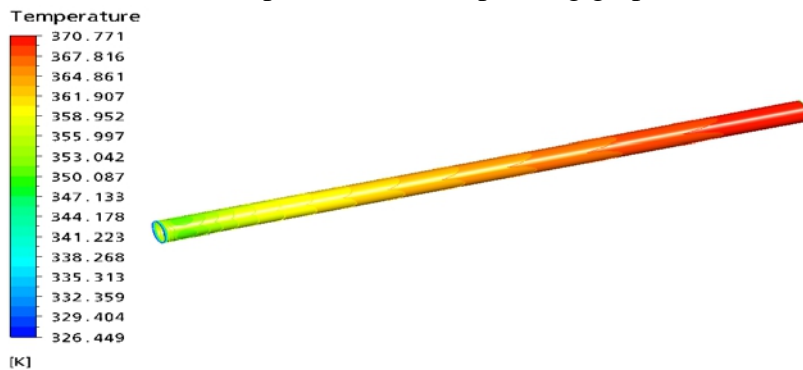
Figures 6: Static Temperature Variations for the Plain Tube configuration on wall
