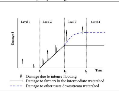
Figure 2. A damage function due to wetland sedimentation
