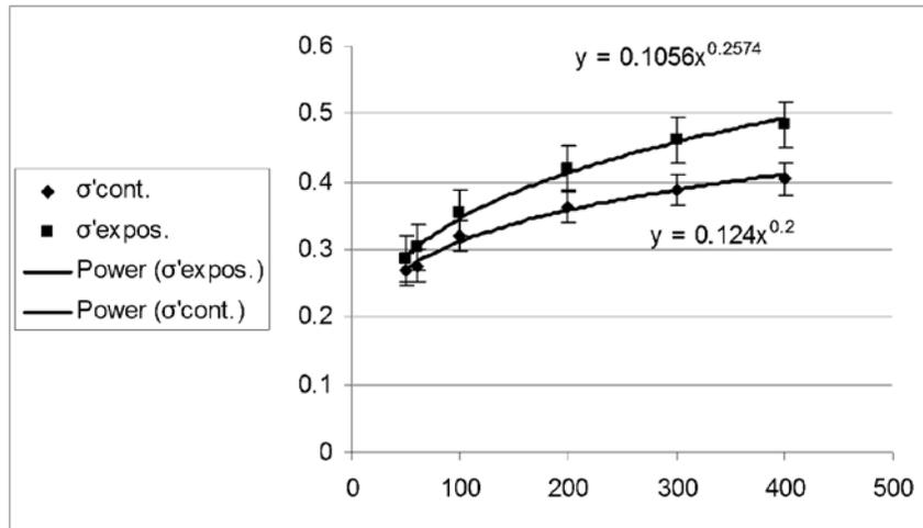
Fig. 2: Variation of the real conductivity  $\sigma'$  (S/m) with frequency  $f$ (Hz) , in the frequency range ( 50 – 400 Hz).
