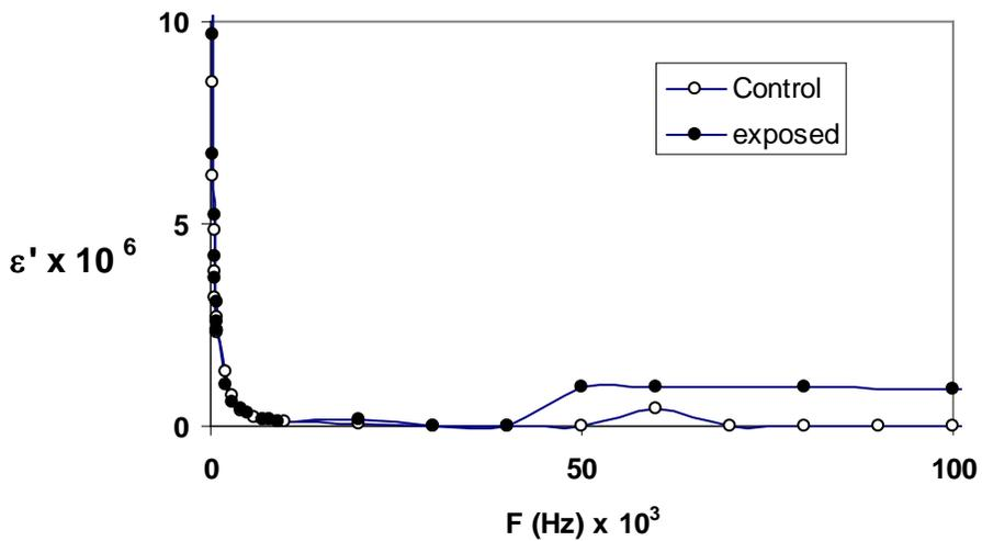
Fig. 3: Variation of the relative permittivity  $\epsilon'$  (F/m) with frequency  $F$  (Hz), in the frequency range (50Hz – 100kHz).
