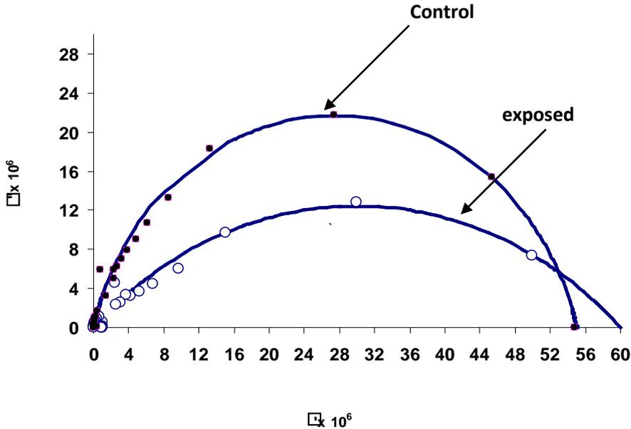
Fig. 10: Cole – Cole diagram between the relative permittivity  $\epsilon'$ (F/m and the dielectric loss  $\epsilon''$  (F/m). Control (●): Exposed (○).
