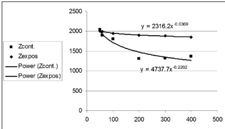
Fig. 6: Variation of impedance Z with frequency f in the frequency range 50 – 400 Hz.
