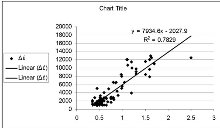
Fig. 8: Correlation between the dielectric increment, expressed as  $\Delta\epsilon'$  and the real conductivity  $\sigma'$ .
