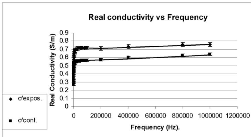
Fig. 1: Variation of the real conductivity  $\sigma'$  (S/m) with frequency  $F$ (Hz) ,in the frequency range ( 50Hz – 1 M Hz).
