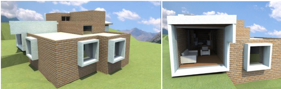
Fig. 8 Views of proposal no. 3: big windows, more modern design, use of adobe, ventilation trough roof opening in corridor.
