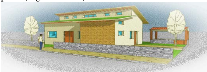
Fig. 6 Home proposal no. 1: small windows for privacy, green roof, exterior areas, stack effect for natural ventilation.
