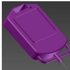
Figure 2 - 10 liter oil reservoir, where oil will be poured to be pumped to the filter and the cleanliness test machine, and then back to the reservoir.
