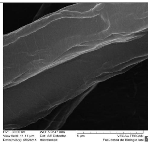
Figure 24. Scanning electron micrograph (SEM) showing absence of microbial load of the paper support (the 1870 printed book) following the treatment with plasma (N<sub>2</sub> atmosphere, 60 seconds)
