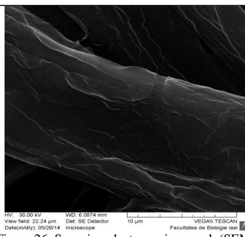
Figure 26. Scanning electron micrograph (SEM) showing absence of microbial load of the paper support (19th century Church book) following the treatment with plasma (N<sub>2</sub> atmosphere, 60 seconds)
