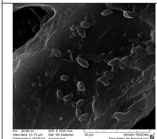
Figure 25. Scanning electron micrograph (SEM) showing microbial load of the paper support (19th century Church book) prior to the treatment with plasma
