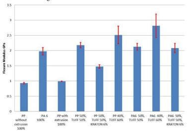
Figure 1. Flexural modulus test results
