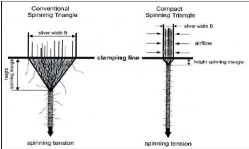
**Figure 2:** comparison of spinning triangles at conventional ring and compact spinning systems (jaswant rajaney,2008,10).
