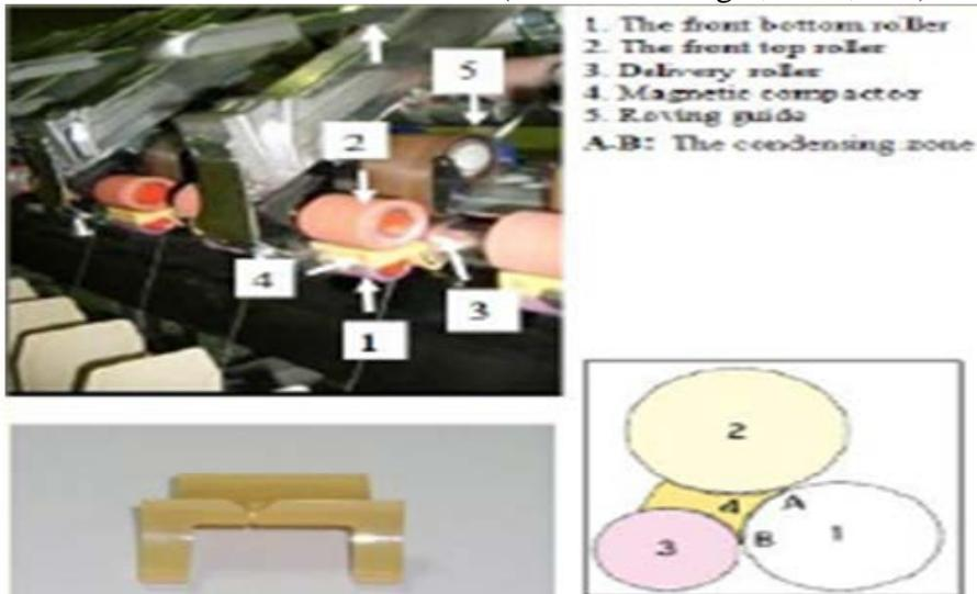
**Figure 3:** The view of rocos mechanical compact spinning and back view of magnetic compactor (Atlas & Kadoglu)
