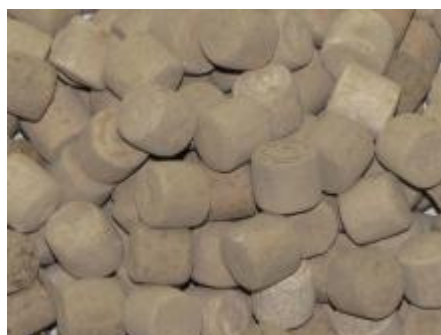
Fig.2 The pellet of ruthenium putting catalyst on the pillar structured montmorillonite
