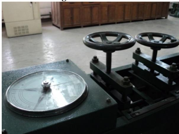
Figure 1. Horizontal tensile strength tester
