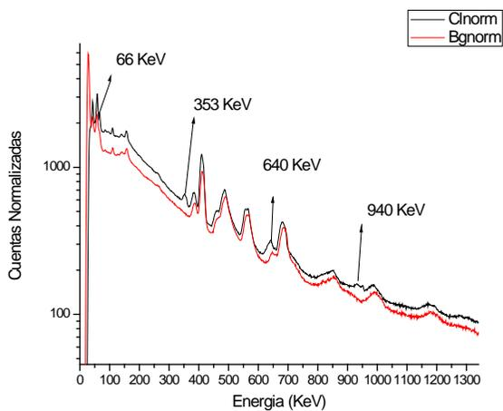
Fig. 5. Gamma spectrum. Sample: chlorine. Low energy.
