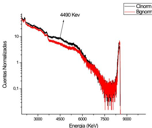
Fig. 7. Gamma spectrum. Sample: chlorine. High energy.
