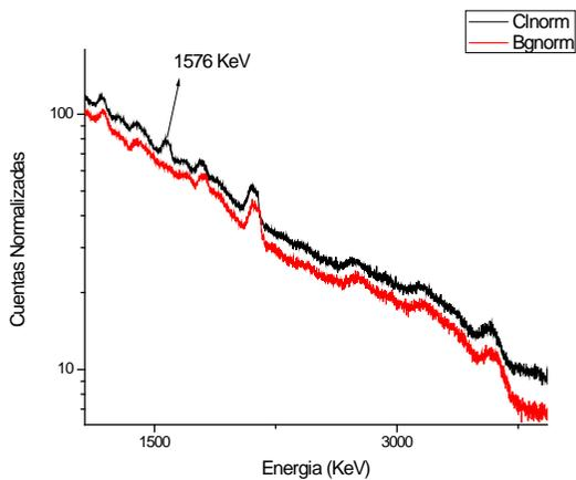
Fig. 6. Gamma spectrum. Sample: chlorine. Intermediate energy.
