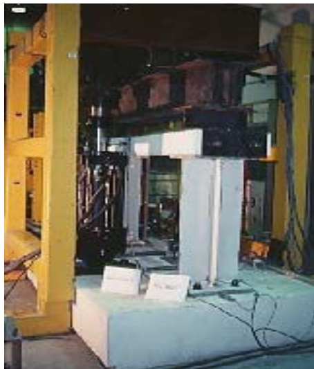
Fig.4 Equipping the test includes placement of loading frames and holders of test samples
