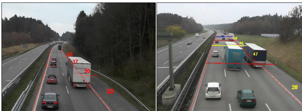
Fig. 5 The A8 motorway near Winkl, 114 km/h, 9 m (0.28 s)
