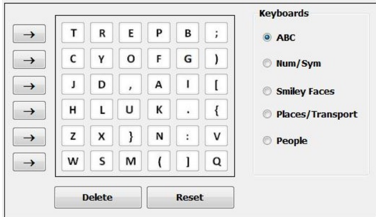
Figure 4: Login session: randomly distribute all characters over the cells of each keyboard
