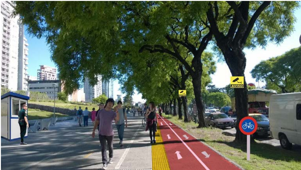
Fig. 17 Proposals for connecting parks. Connector linear park in Buenos Aires city: painting the pavement can create a better division between new bicycle lanes and pedestrian areas. The presence of guards is advisable to help maintain the security of the corridor.
