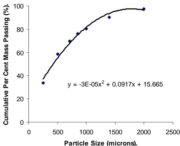
**Figure 2:** Reference ore (quartz) discharge, particle size analysis
