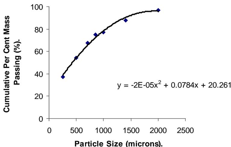
Figure 3: Lead-gold ore discharge particle size analysis.
